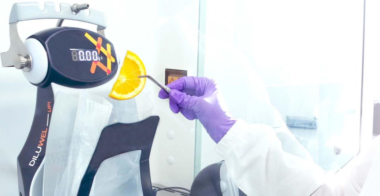
DILUWEL UP! is a fast, robust & accurate gravimetric dilutor, that dilutes solid samples with the correct amount of diluent in few seconds.
